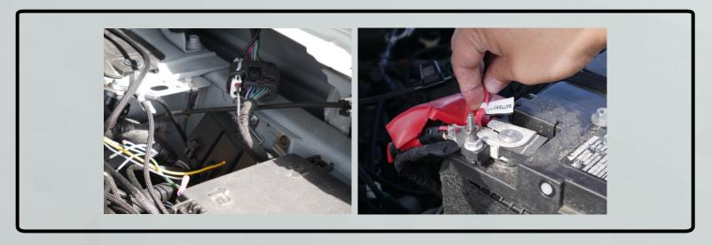
12. Using a butt connector, connect the harness's trigger wire to the upfitter switch using the appropriate wire (which can be found in the owner's manual).
