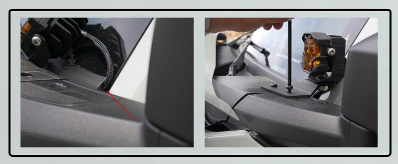
10. Adjust pod angle and direction. Fully tighten the fasteners using the TP30 (torx plus) socket or L-key.
