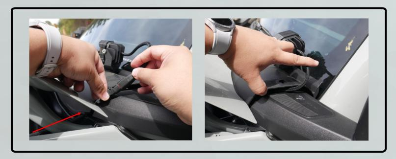
8. Run wire behind trim panel and under the recess left from Ford. This will ensure the cable is not pinched once installed.
