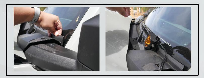
7. Run cable up from the engine bay and under the trim piece that was just loosened. Connect Deutsch connector to 4Banger pod. Begin tucking wire under loose trim panel and begin routing wire up towards the top corner.
