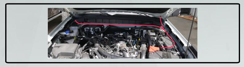
6. Lift trim. Starting with the corner that sits against the glass, lift straight up until the cowl is released from its groove. Now pull up on the trim piece near the hood to loosen the panel. Trim only needs to be loosened in the corner, not removed. Place assembled 4Banger Pod on cowl near windshield wiper with cable facing the mirror.
