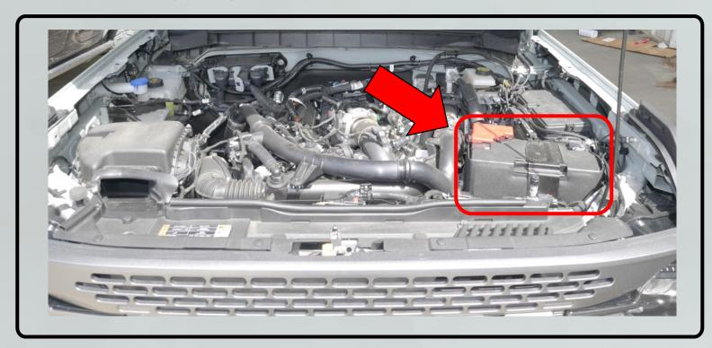
2. Using a 10mm socket or wrench, loosen the nut holding the negative battery terminal to the battery. Note: The nut only needs to be loosened, <u>not</u> removed. Remove the battery terminal and set safely aside
