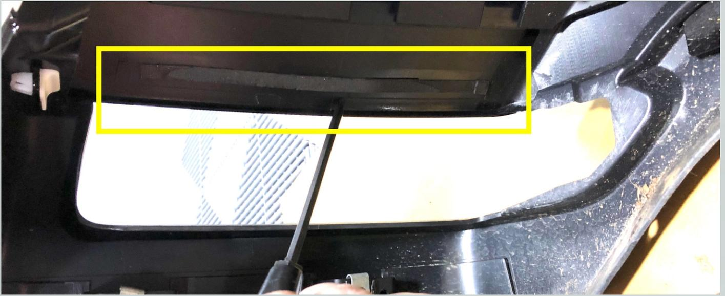
10. Remove the OEM wire harness for the stock DRL that runs to the back of the fender. There are a couple clips holding it in. Then re-route the harness for the new LED DRL back in the same place.
