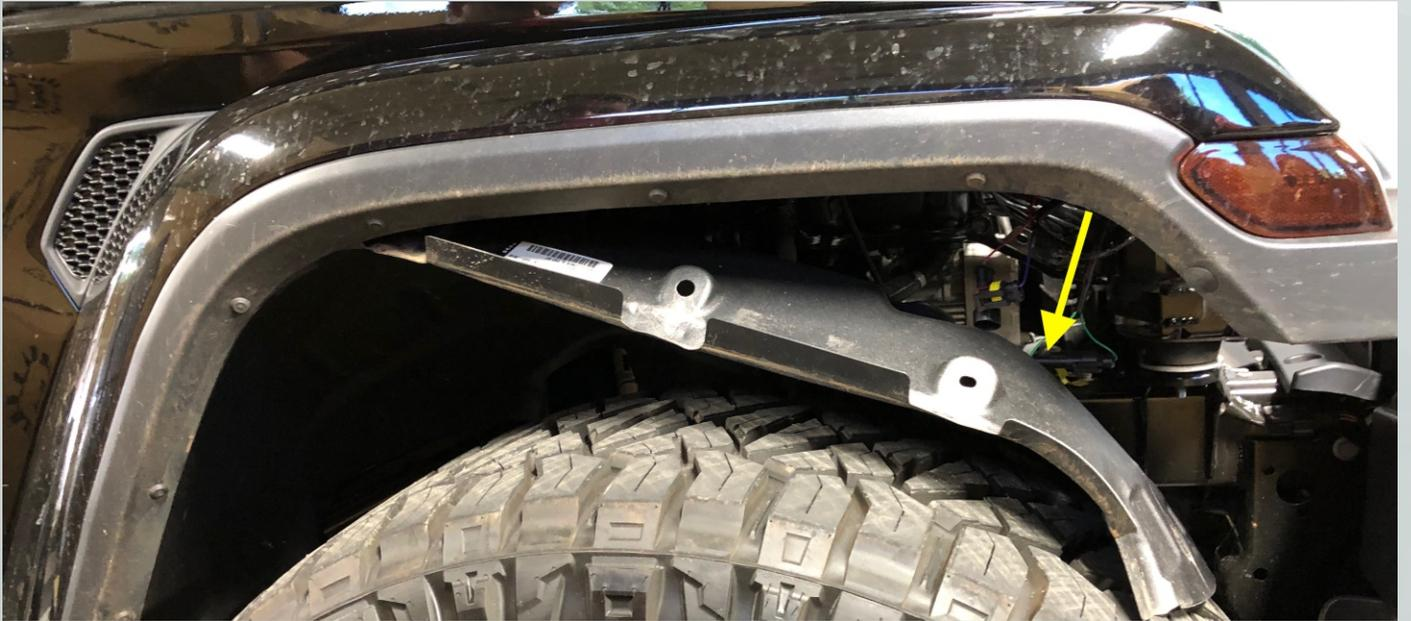
2. Lift the entire fender up and away from your Jeep. There are several clips holding it on as you can see from the images below, but you can pull it off with moderate force to safely remove it.
