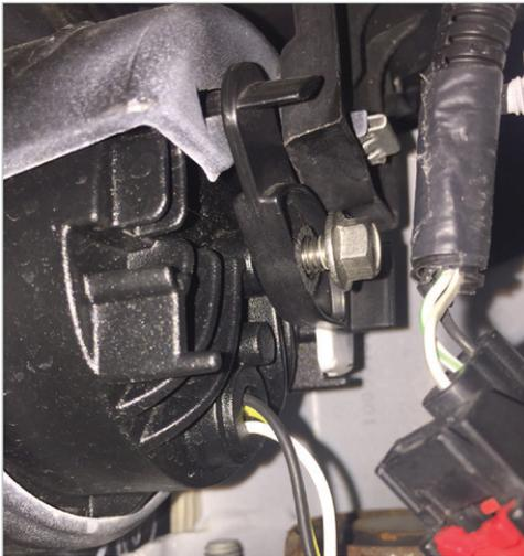
7. Insert the Model 239 J2 connector into the vehicle's connector. **You must lock the connectors together** by pushing the red retaining lock toward the turn signal connector, as shown.
