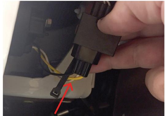
2. Loop the zip tie around the vehicle connector, passing through the wires. Close the zip tie to secure the two connectors.
