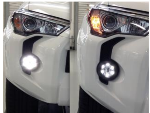
Left: showing LED Fog Light "ON" Right: Showing DRL "on"
