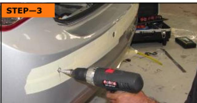
Using masking tape, measure the rear bumper for even positioning of the sensor heads. Once accurate, drill holes for the sensor heads.
