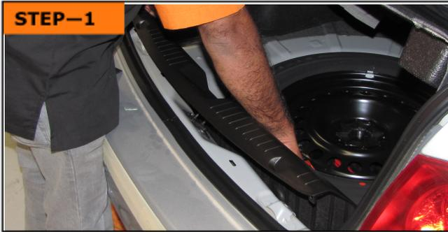
Using Plastic tool, remove rear trunk trim.
