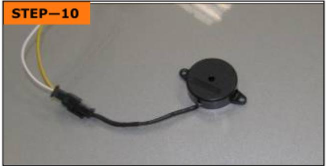
Connect the buzzer. Using the double sided tape, place buzzer in the trunk, in a hidden position. Position the buzzer so it can be heard well from the driver seat.
