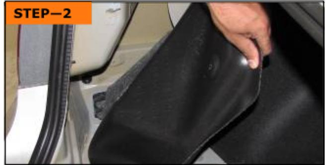
Using plastic tool, remove left side interior panel to reveal reverse light connection.
