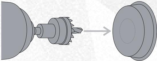
Your factory housing cap must be drilled with a 20mm / 0.75" hole saw for the grommet to fit snugly in the cap.
